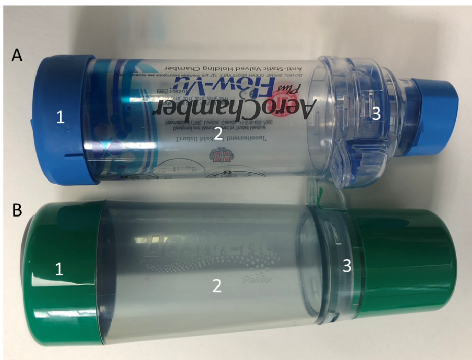
Figure 1 Anti-static VHC devices tested: AeroChamber Plus Flow-Vu™ (A) and DosiVent® (Palex Medical) (B). 1) indicates the inhaler adaptor, 2) the VHC and 3) the rubber valve close to the mouthpiece.
